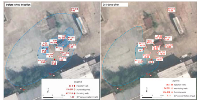
Kortan site - Cr(VI) concentrations in groundwater before and after substrate application
