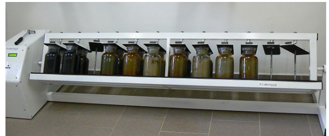
Laboratory batch test of bio-reduction potential
