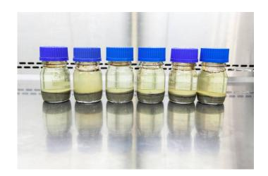
DEKONTA performs batch or column tests to simulate chemical oxidation of various types of contaminants (BTEX, petroleum hydrocarbons, CVOCs, MTBE and others), to evaluate the requirements that help in proposing the technology design:
