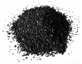
The regeneration is carried out with superheated steam at temperatures up to  $350\,^{\circ}$  C. This allows a thermal desorption of the GAC without pyrolysis or combustion, therefore no burnout or opal GAC is produced and the porous surface area is not damaged, thus the performance of the regenerated GAC remains the same. Our system is able to treat 500 kg of GAC in a 8 hours shift! The unit consists of one 20' and a 40' containers.
