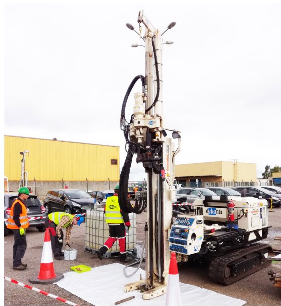
High pressure direct push application of whey using drilling rig Geoprobe 7822 dt
