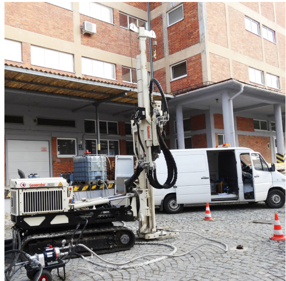
High pressure direct push application of nanoscale ZVI using drilling rig Geoprobe 7822DT
