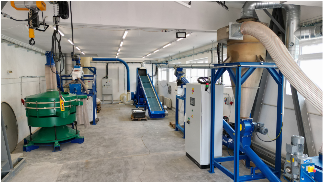
Line for recycling waste photovoltaic panels
